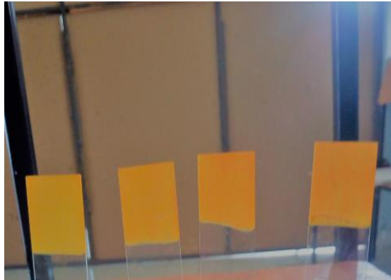
Figure 4.7: The Color of CdS thin film after deposition at t= 45, 60, 75,90min respectively.
